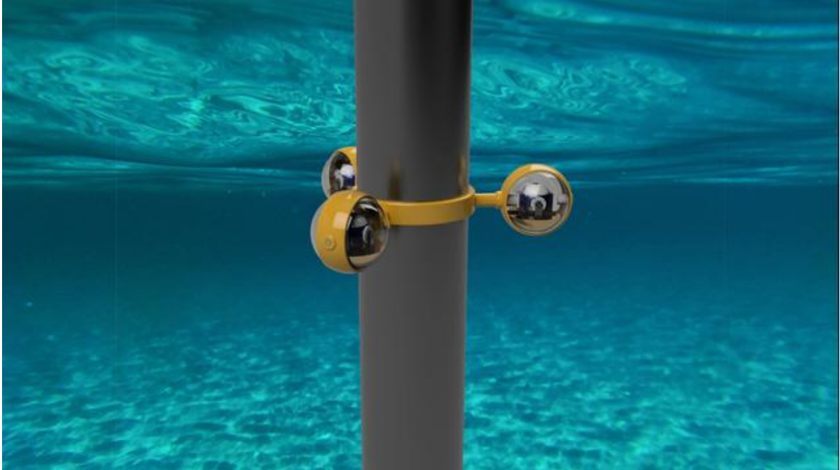
Figure 5 – WITT Suggestion for Riser Damping Configuration
